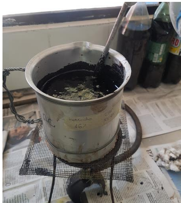
Figure 3. Incorporation of rubber into CAP.
