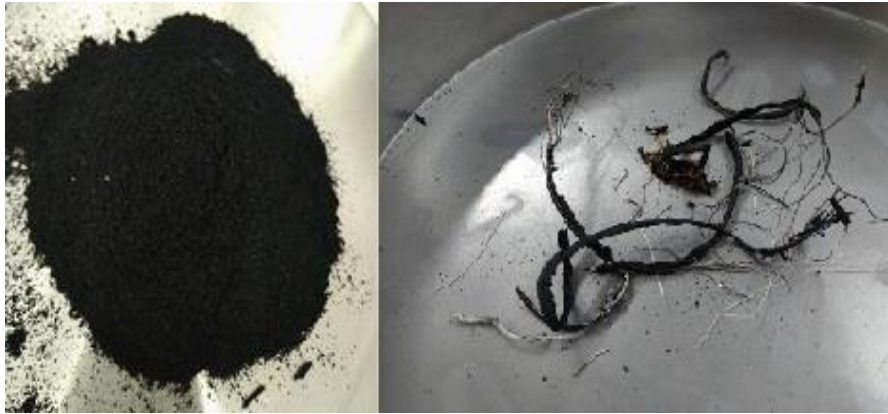
Figure 1. Ground rubber used (left) and Impurities (right).
