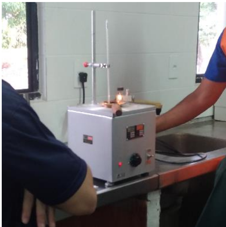
Figure 6. Checking for the release of flammable gases.
