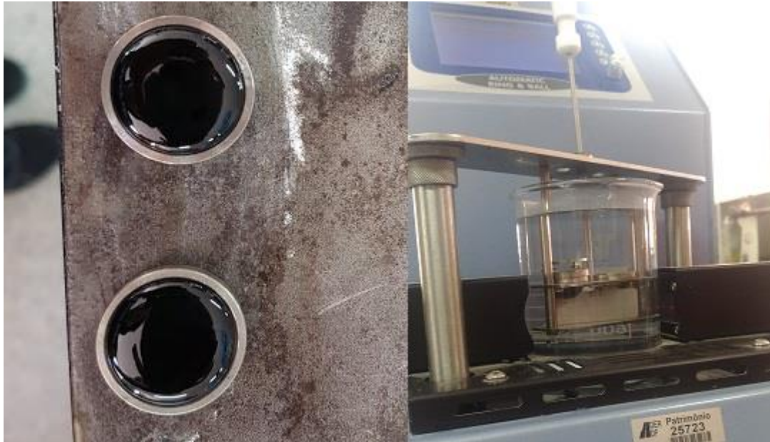
Figure 4. Test specimen (left) and apparatus (right) for the Softening Point test.
