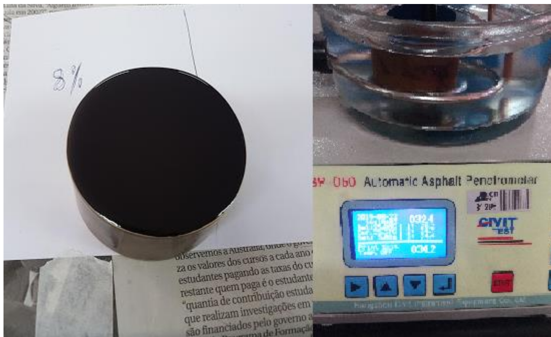
Figure 5. Mold for the Penetration test (left) and its respective results (right).
