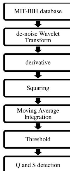
Figure 2. Block Diagram of Method 3
