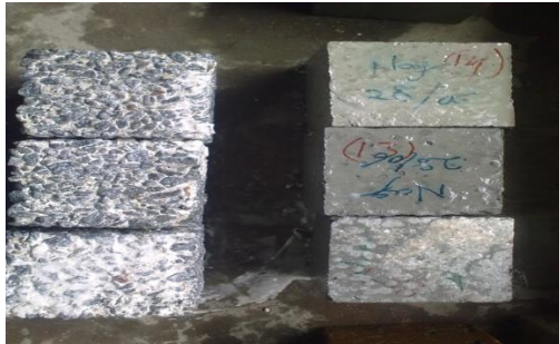
Fig:7 Concrete cubes after acid immersion in H 2 SO 4
