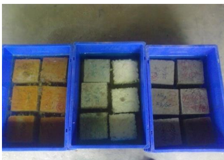
Fig:5 Immersion of concrete cubes
