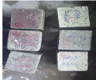
Fig:8 Concrete cubes after immersion in MgSO 4
