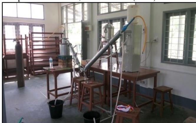
Figure 2. Experimental setup for fuel oil production process
