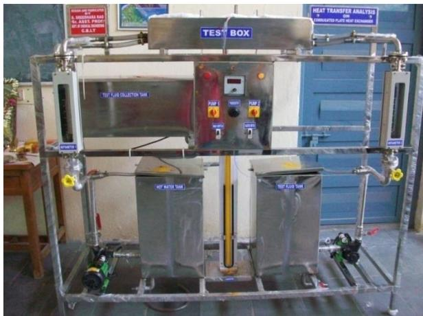
**Fig -1:** Plate heat exchanger setup.
