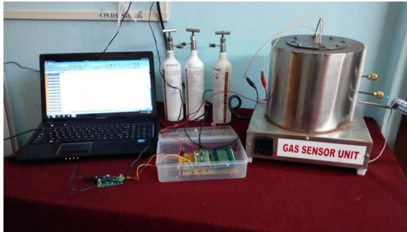
Fig.8 Experimental setup for the calibration of ARM based CO gas monitoring system
