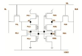
Figure 2: The 10T SRAM Cell
