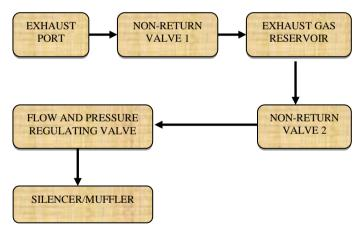
Figure 2: Diagrammatic Representation of the Process **Note**: Valves used here are pneumatic valves of suitable size and configuration
