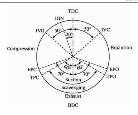
Figure 3: Port Timing Diagram of Two Stroke Engines
