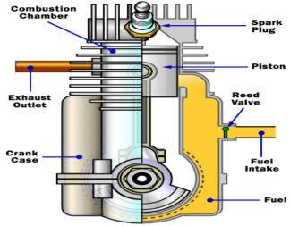
Figure 1: Two Stroke Engine Components
