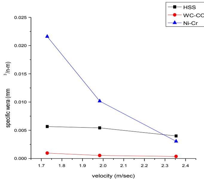
Figure 5. Effect of speed on specific wear rate for various compositions
