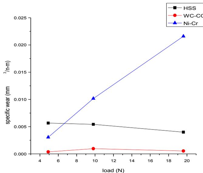
Figure 6. Effect of normal load on specific wear rate for various compositions
