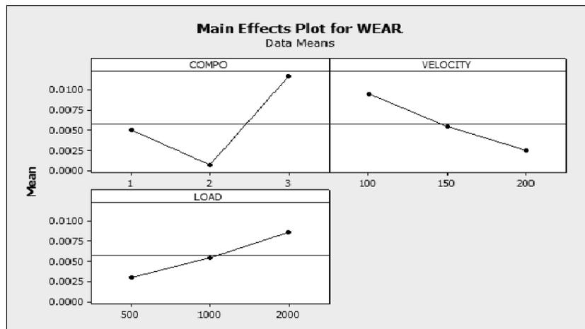
**Figure 4.** Effect of control factors on wear rate
