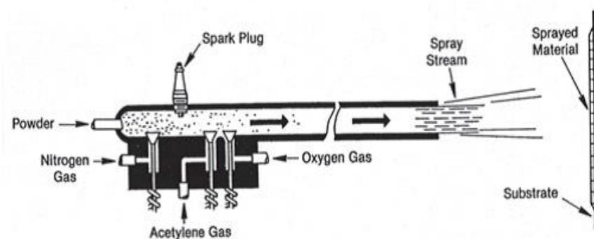
**Figure 1.** Schematic of Detonation Gun Process
