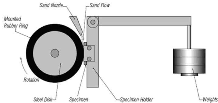
**Figure 3.** Dry Sand Rubber/Wheel Abrasion Test
