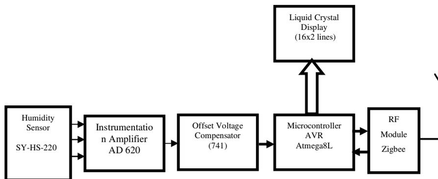
Figure 1 Block diagram of the Wireless Sensor Node for WSN for Polyhouse applications
