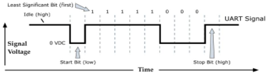
Figure 8. UART data packet 0x1F as transmitted through the RF module
