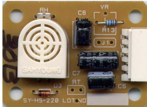
Figure 3: Humidity Sensor SY-HS-220
