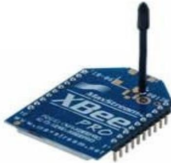
Figure 6. RF Module The Zigbee Pro
