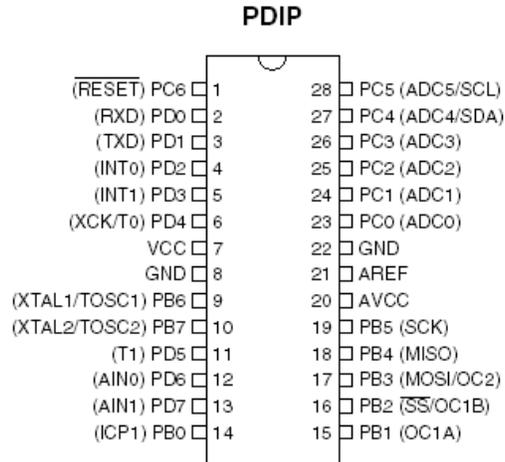
Fig.5: Pin description of AVR Atmega8L
