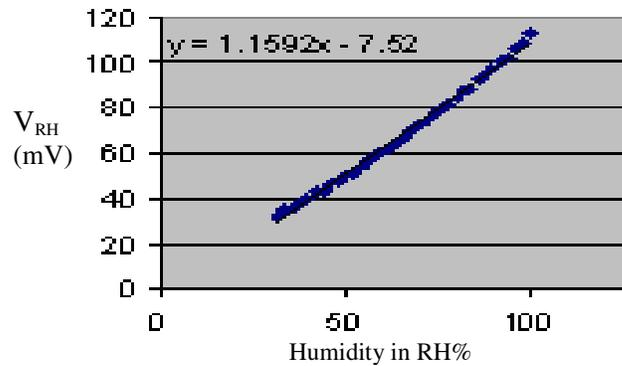
Figure 10: Graph of observed emf (mV) against applied humidity in RH%
