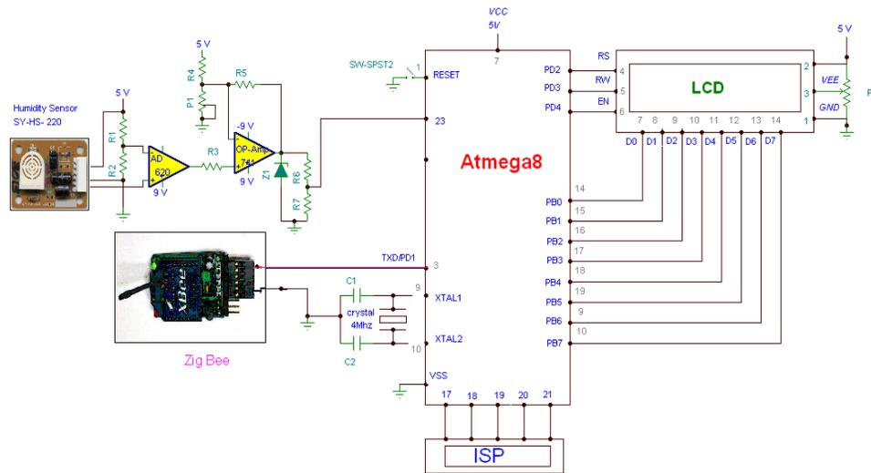
Figure 2.a: The schematics of the circuit of the wireless sensor node.
